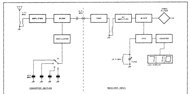
fig. 1. Conversion scheme of the GP-63/GP-60 converter/receiver combination. Set tunes the 2.0-3.0 MHz band and receives on 11.71 MHz.
